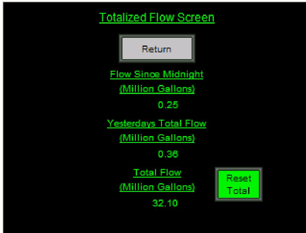
The **Totalized Flow Screen** displays real time data for the pump station flow for three different timeframes: the current flow since midnight; the total flow for the last day (24 hour period) and the total flow to date. Use the reset button to clear the totals to get data for a new period of time. All data is displayed in digital readouts up to the second decimal point.
