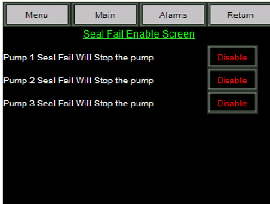
The **Seal Fail Enable Screen** directs your system whether or not to stop the pumps when a Seal Failure occurs. When the “Pump 1, 2 or 3 Seal Fail” Button is ENABLED, the pump will stop when a seal fail occurs. If the button for Pump 1, 2 or 3 is disabled, the alarm will occur, but the pump will continue to run.
